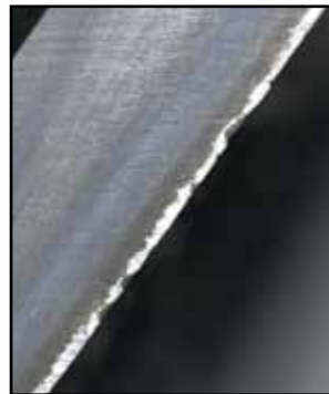
OSG's VGx®-5: Mild Chipping; Good Wear
