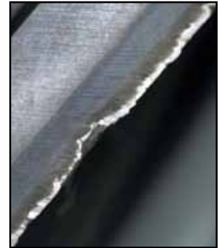
Competitor: Severe Chipping; Large Wear
